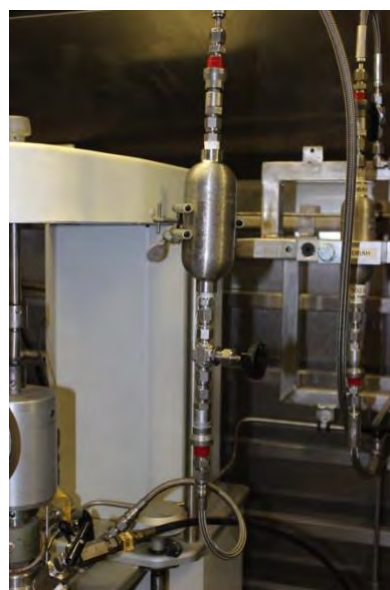
Fig-6. Catalyst & Scavenging Dibah charging to reactor
